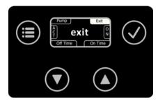
Bottom left the waiting time can be set in 0.1 minute (6 sec.) steps. Analogously, the fogging time can be set in steps of seconds at the bottom right. To activate the timer, the confirmation key can be pressed for both the waiting time or the fogging time. This activates or deactivates the timer. Depending on the selected menu item, the timer starts with the waiting time or the fog time.
