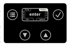
value field. The confirmation key is used to access the submenu for Modbus.
