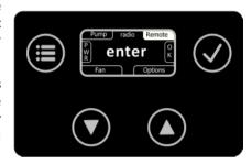
Up to 60 different handheld transmitters can be programmed on the machine. For this purpose, the "Remote" submenu must first be selected.
