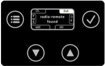
menu item add and confirm this with the confirmation key. "Adding" now appears at the bottom left. The machine now waits for a valid radio signal. To do this, press any key on the handheld transmitter. The teach-in process is now complete and "adding" appears again at the bottom left. You can then select the key and save it.
